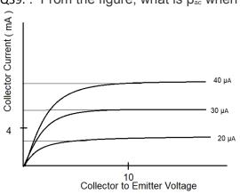
Q39. . From the figure, what is  $\beta_{ac}$  when  $V_{CE}$  is 10V and  $I_c$  is 4 mA?
